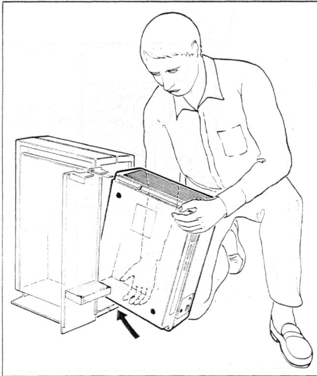
**Step 2.** Slide the system unit into the floor stand.
