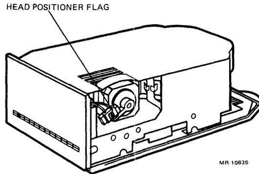
Figure 6-3 RD51 Disk Drive Head Positioner Flag
