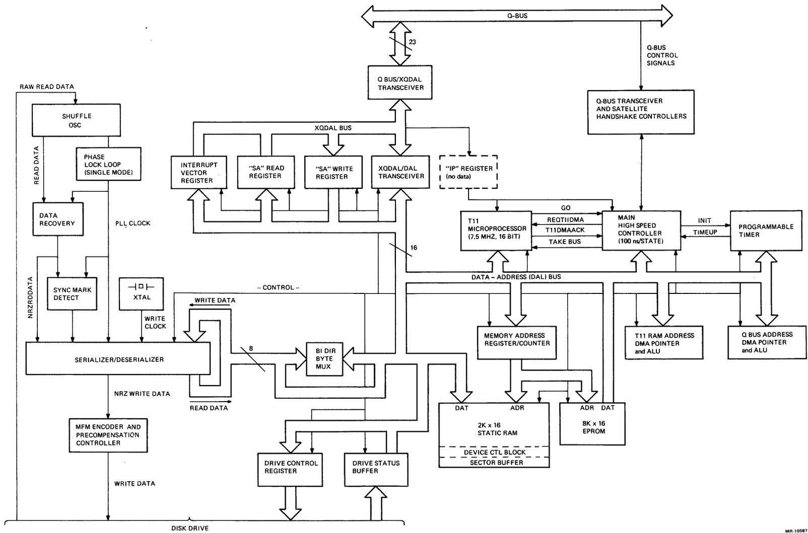
Figure 2-1 RQDX1 Controller Module Functional Block Diagram
