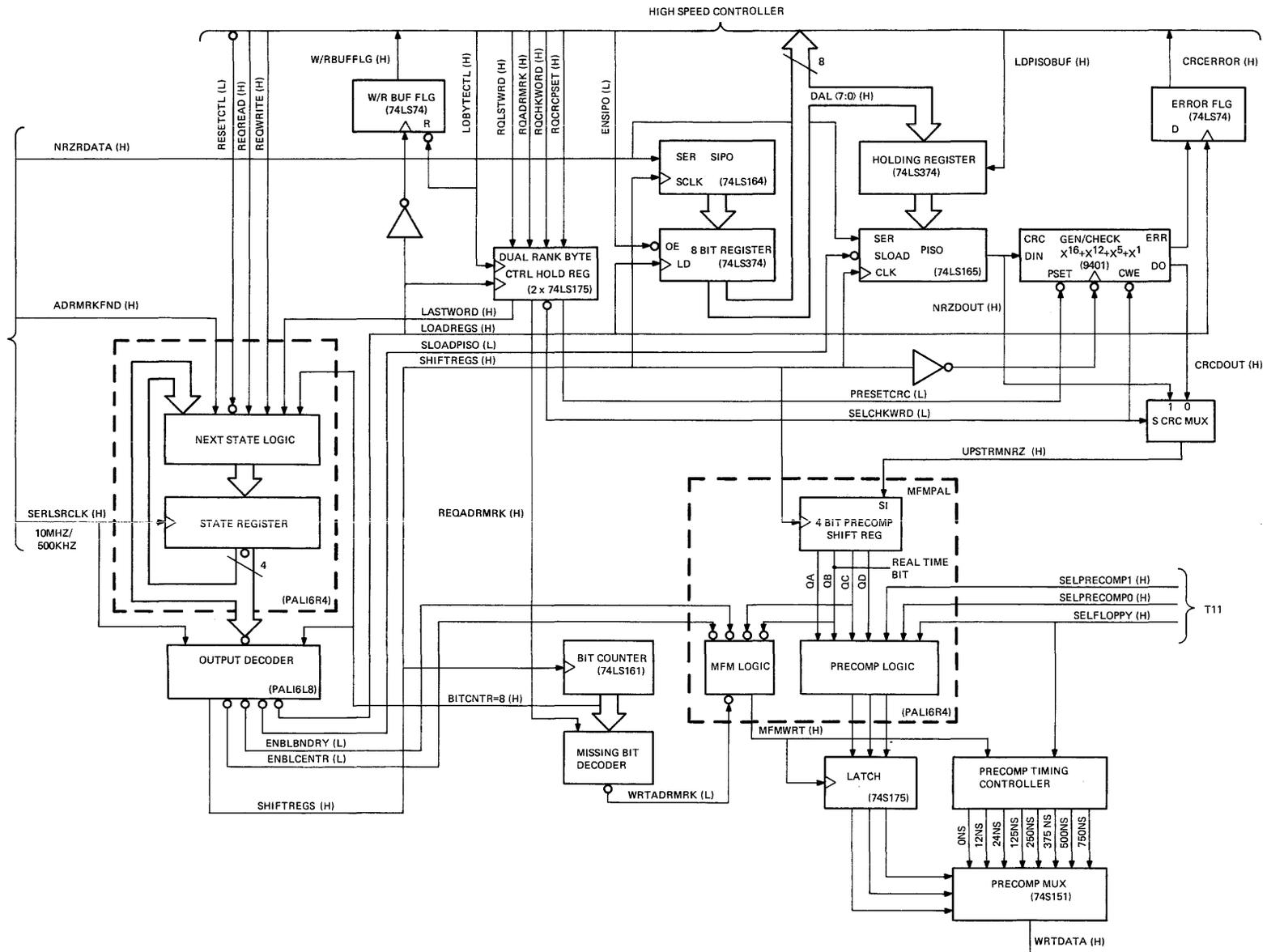
Figure 2-5 Serializer/Deserializer and MFM Encoder/Precomp Generator Logic
