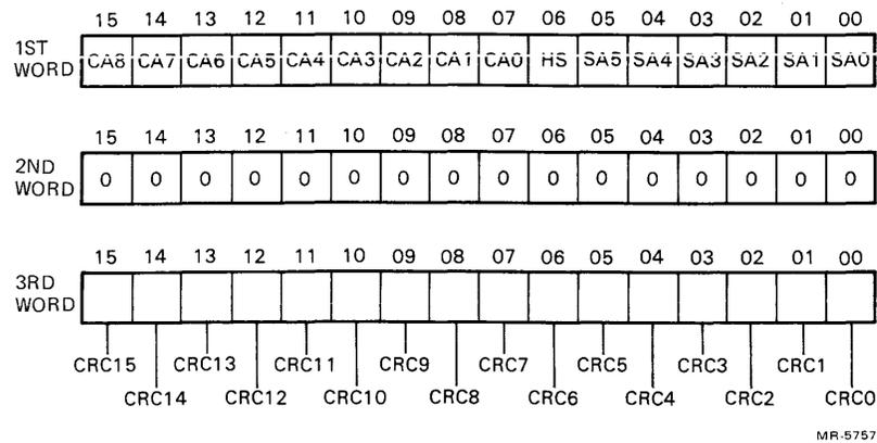
Figure 4-7 Reading the MPR After a Read Header Command (Three Header Words)
