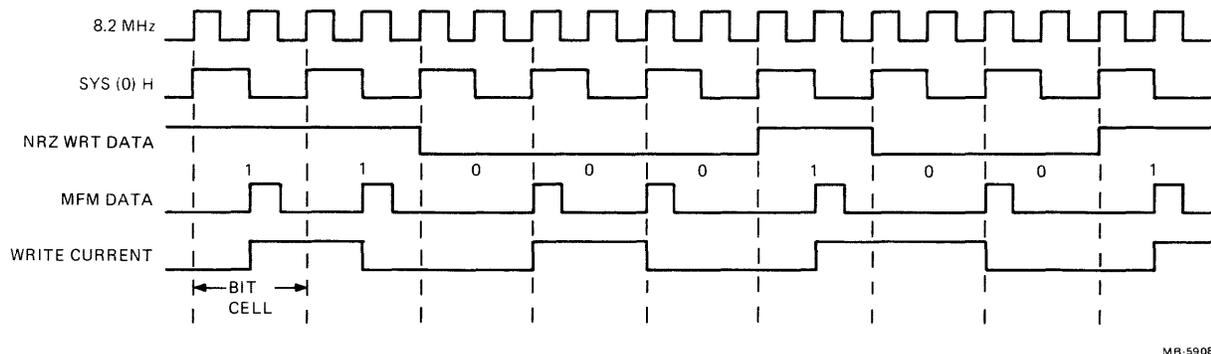
Figure 2-10 MFM Encoding
