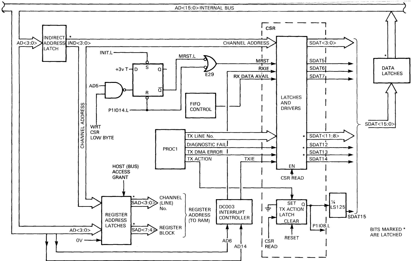
Figure 4-20 CSR and Register Address Circuits
