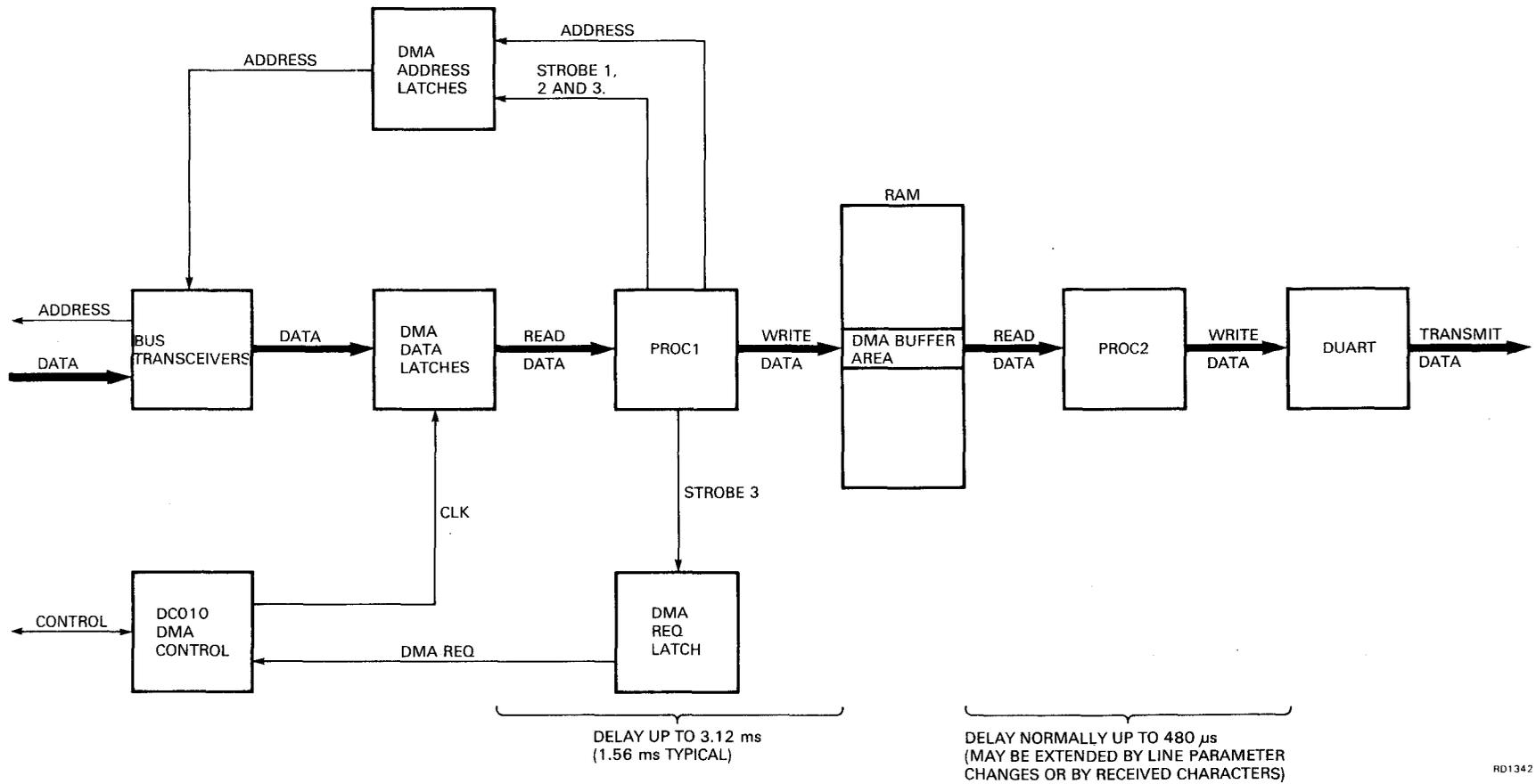
Figure 4-11 DMA Data Transfer
