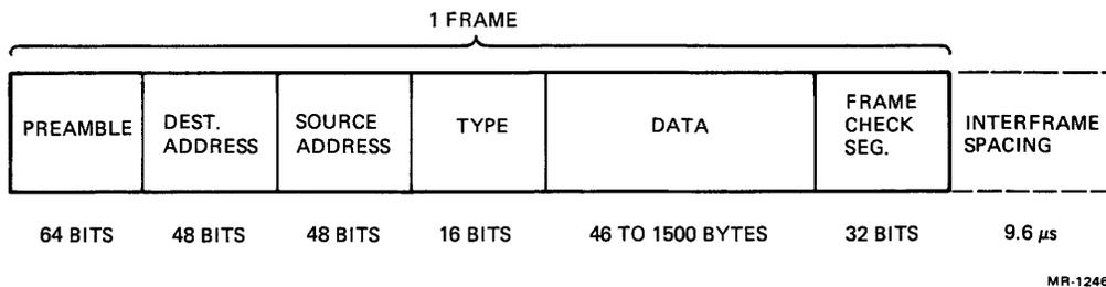
Figure 1-3 ETHERNET Packet (Frame) Format
