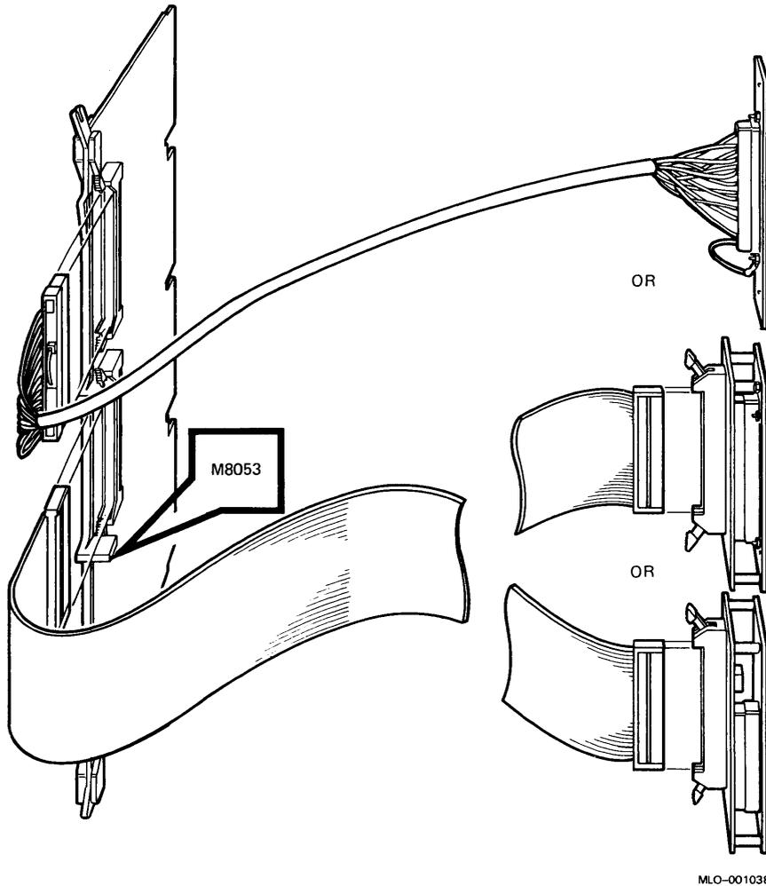
Figure 4: DMV11-N Internal Cabling (M8064)
