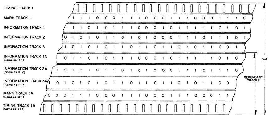
Figure 2-2 Track Allocation Showing Redundantly Paired Tracks
