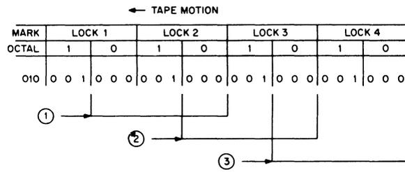
Figure 3-7 Mark-Track Decoding (MK BLK START-010)
