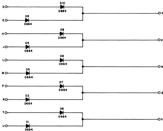
Figure 5-4 R002 Diode Network
