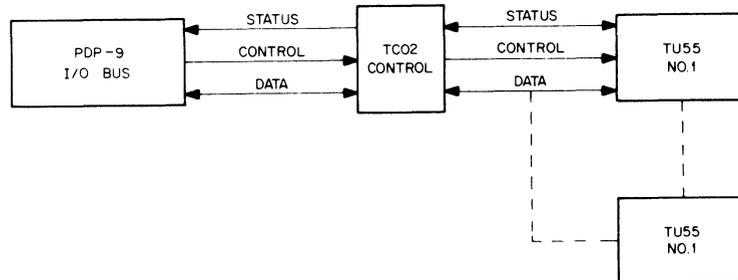
Figure 1-1 System Configuration
