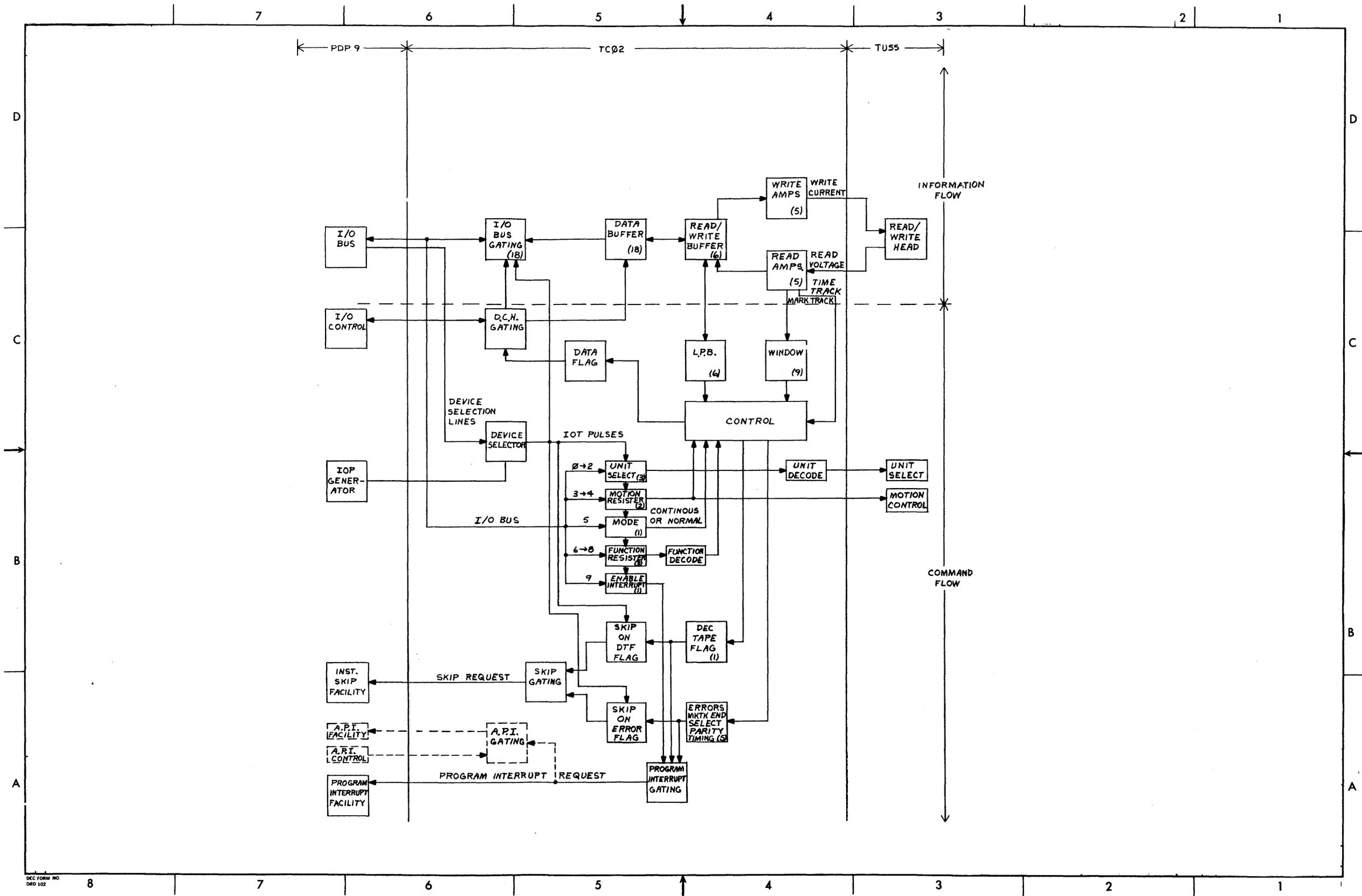
Figure 3-2 Type TC01 DEctape Control Functional Block Diagram
