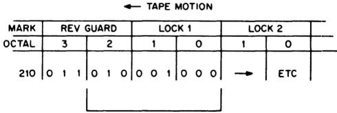
Figure 3-6 Mark-Track Decoding (MK BLK START -210)
