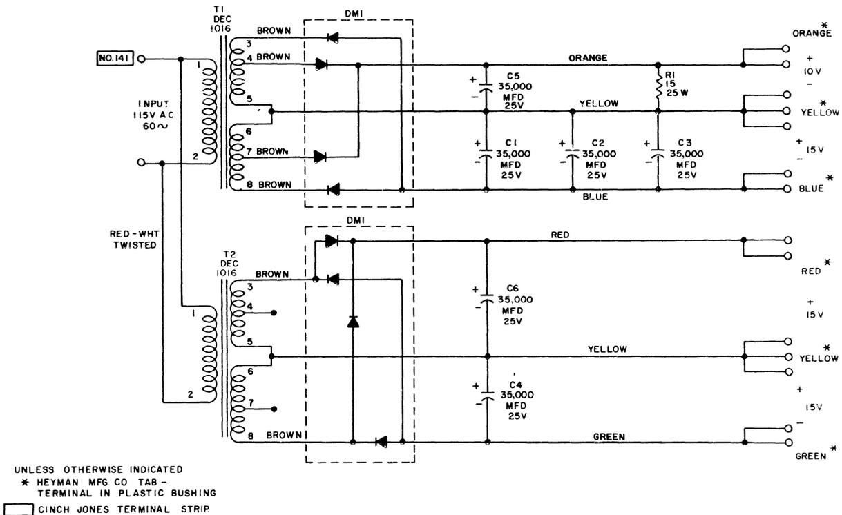
Figure 5-25 Power Supply Type 779, Schematic Diagram
