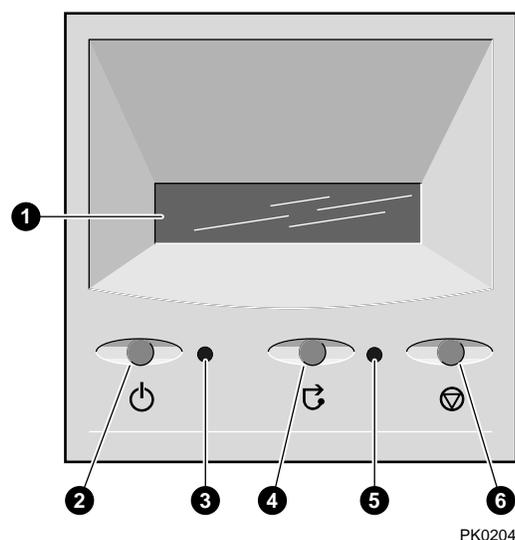
❶ Control panel display. A one-line, 16-character alphanumeric display that indicates system status during power-up and testing. During operation, the control panel is back lit.
