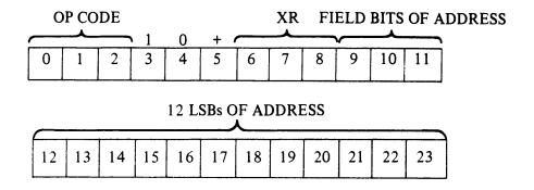
IF XR=0, Y=15-BIT ADDRESS AS GIVEN. THE CONTENTS OF INDEX REGISTER 0 ARE INCREMENTED IF BIT 5 IS LOGIC 1, BUT ARE NOT USED AS PART OF THE ADDRESS CALCULATION.
