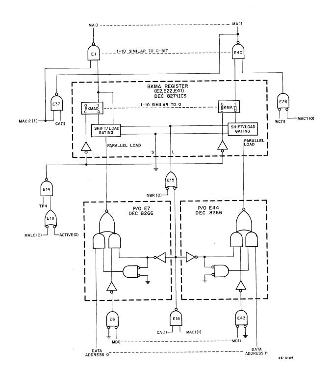
Figure 3-5 BKMA Register Logic
