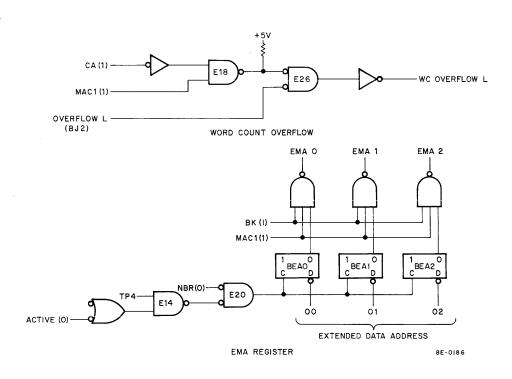
Figure 3-7 Word Count Overflow and EMA Register Logic
