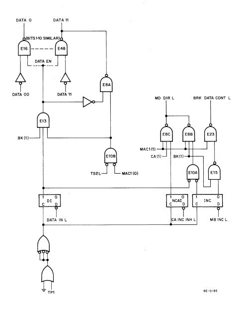
Figure 3-6 Data Transfer Logic
