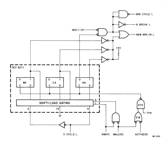
Figure 3-2 Cycle Select Logic
