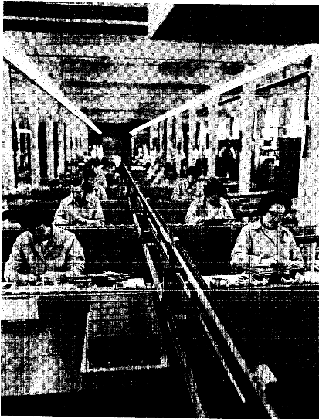
FLIP CHIP assembly line combines automated manufacturing steps with computer controlled checkout for lower cost, more reliable circuits.
