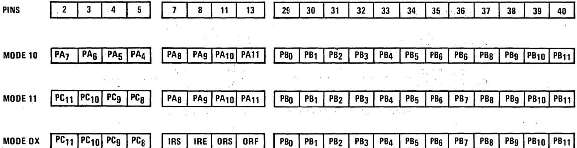
FIGURE 7: IM6103 PIO port pin assignments.
