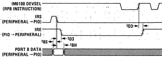
FIGURE 4: Input data transfer (peripheral device to PIO).
