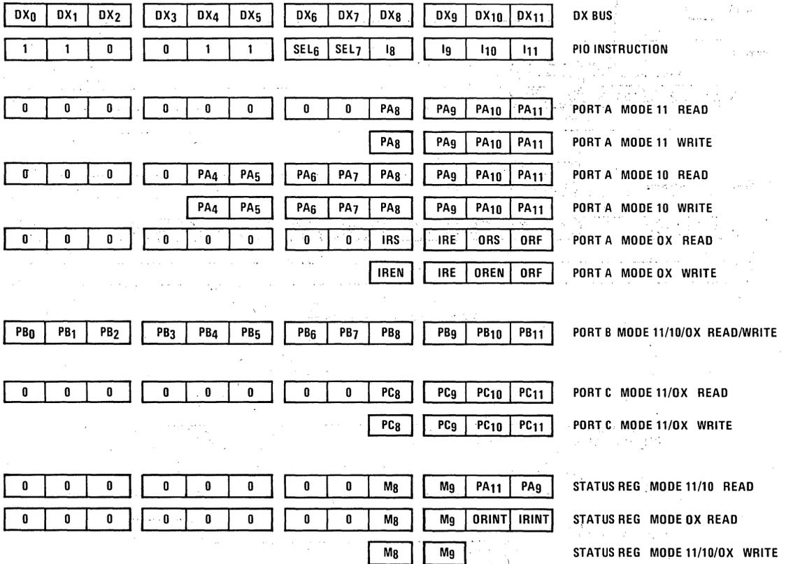
FIGURE 6: IM6103 PIO register bit assignments.
