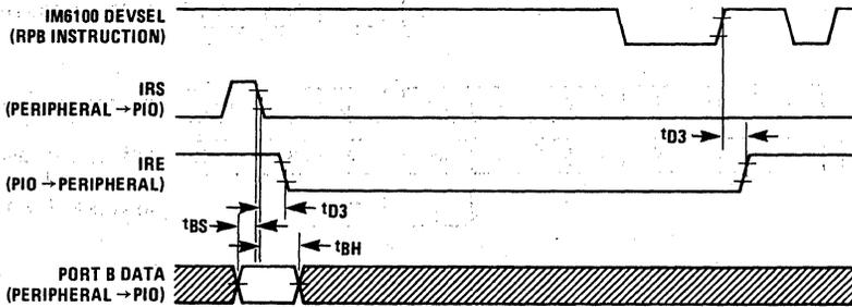
FIGURE 11: Input data transfer (peripheral device to PIO).
