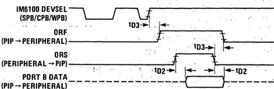
FIGURE 5: Output data transfer (PIO to peripheral device).
