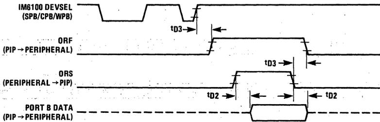
FIGURE 12: Output data transfer (PIO to peripheral device).
