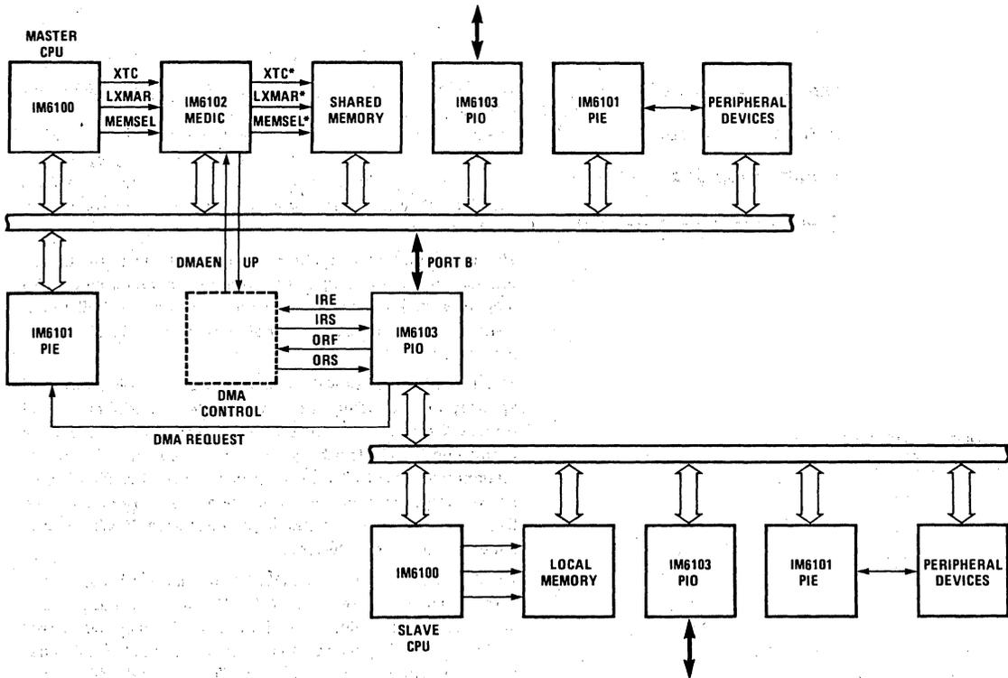
FIGURE 13: Dual processor system with shared memory.
