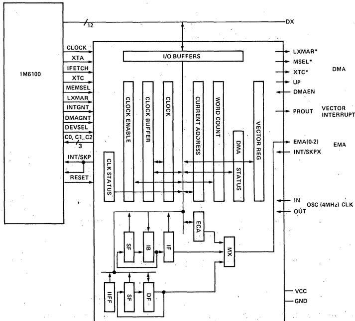
FIGURE 1: IM6102 MEMORY EXTENSION/DMA/INTERVAL TIMER CONTROLLER (MEDIC)
