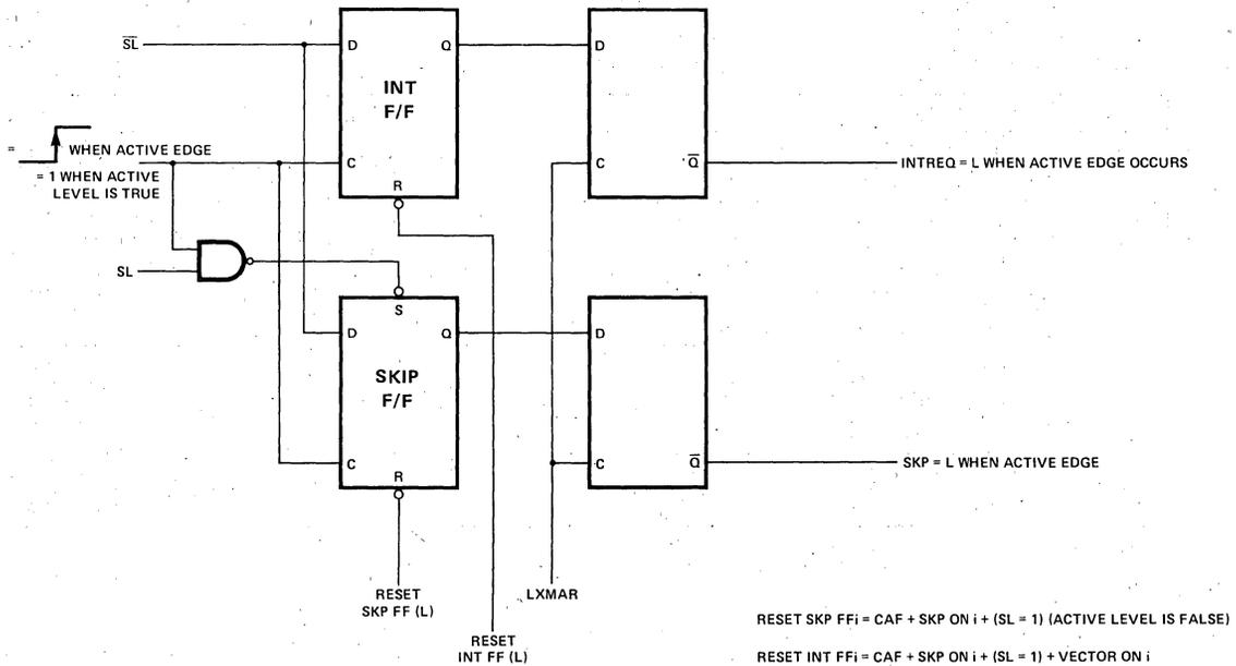
Figure 7. IM6101 SKIP Flip Flop and INTERRUPT Flip Flop Input Diagram.
