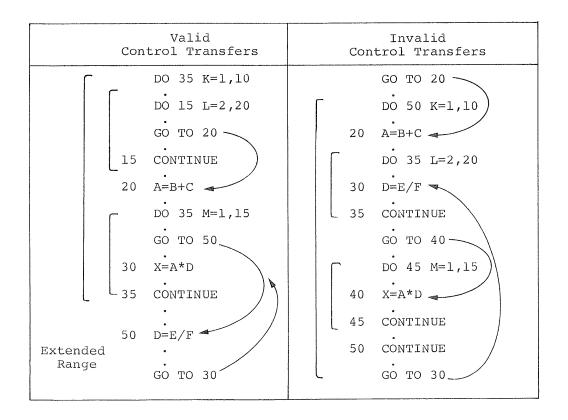
Figure 4-2 Control Transfers and Extended Range
