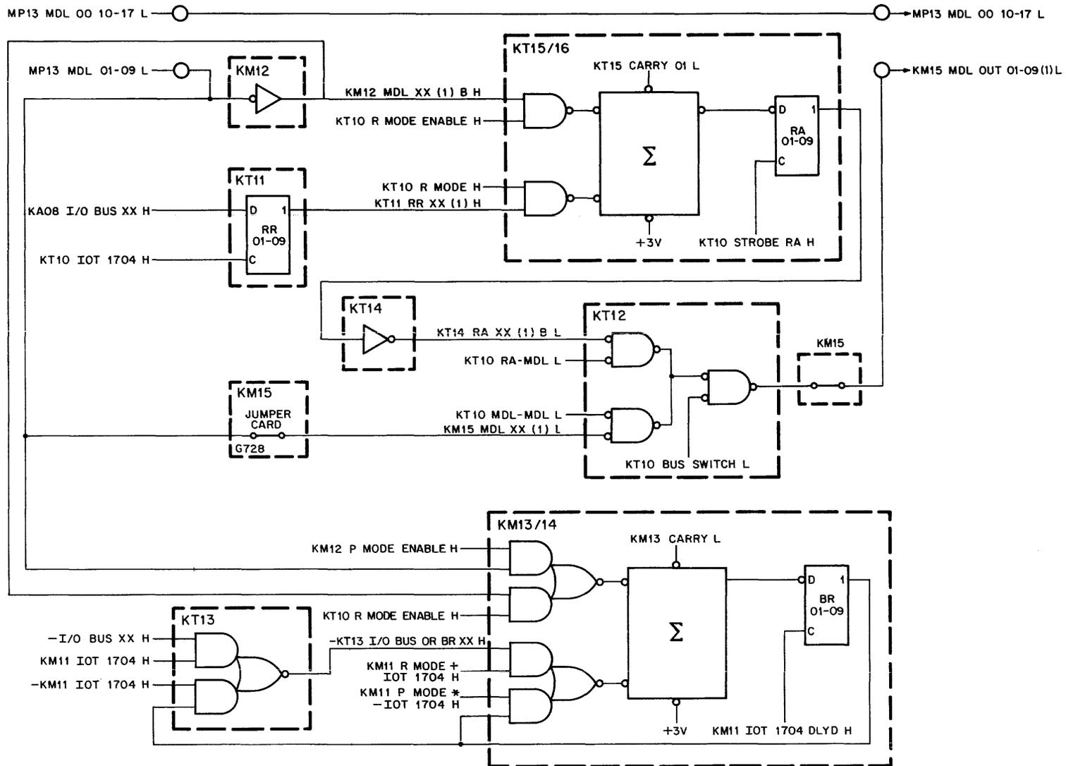
Figure 6-14 Memory Protect and Relocate Interconnection Diagram
