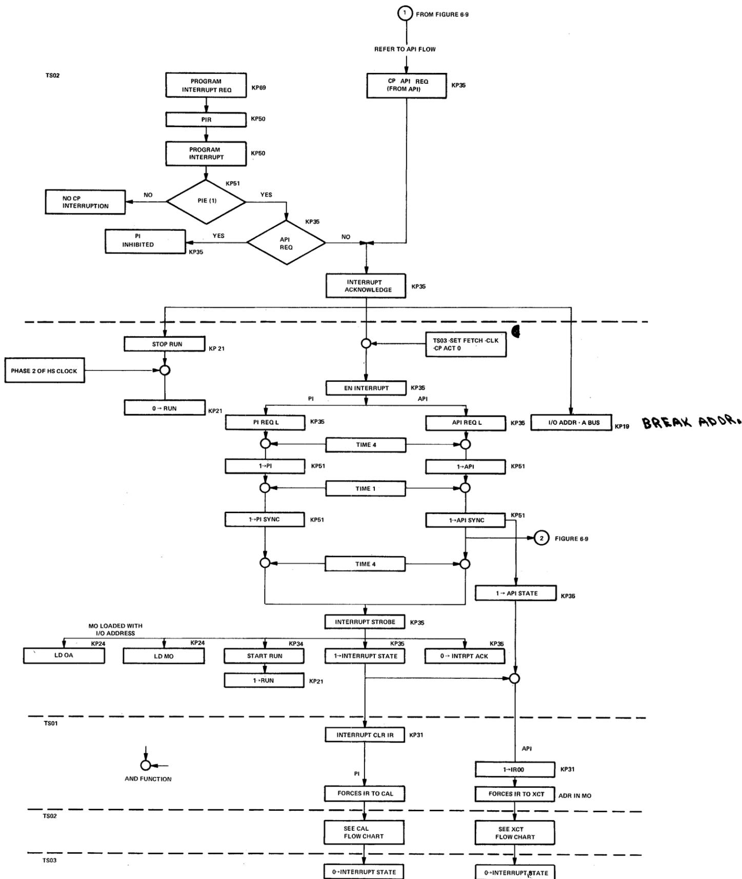
Figure 6-11 API/PI/Central Processor Flow Diagram
