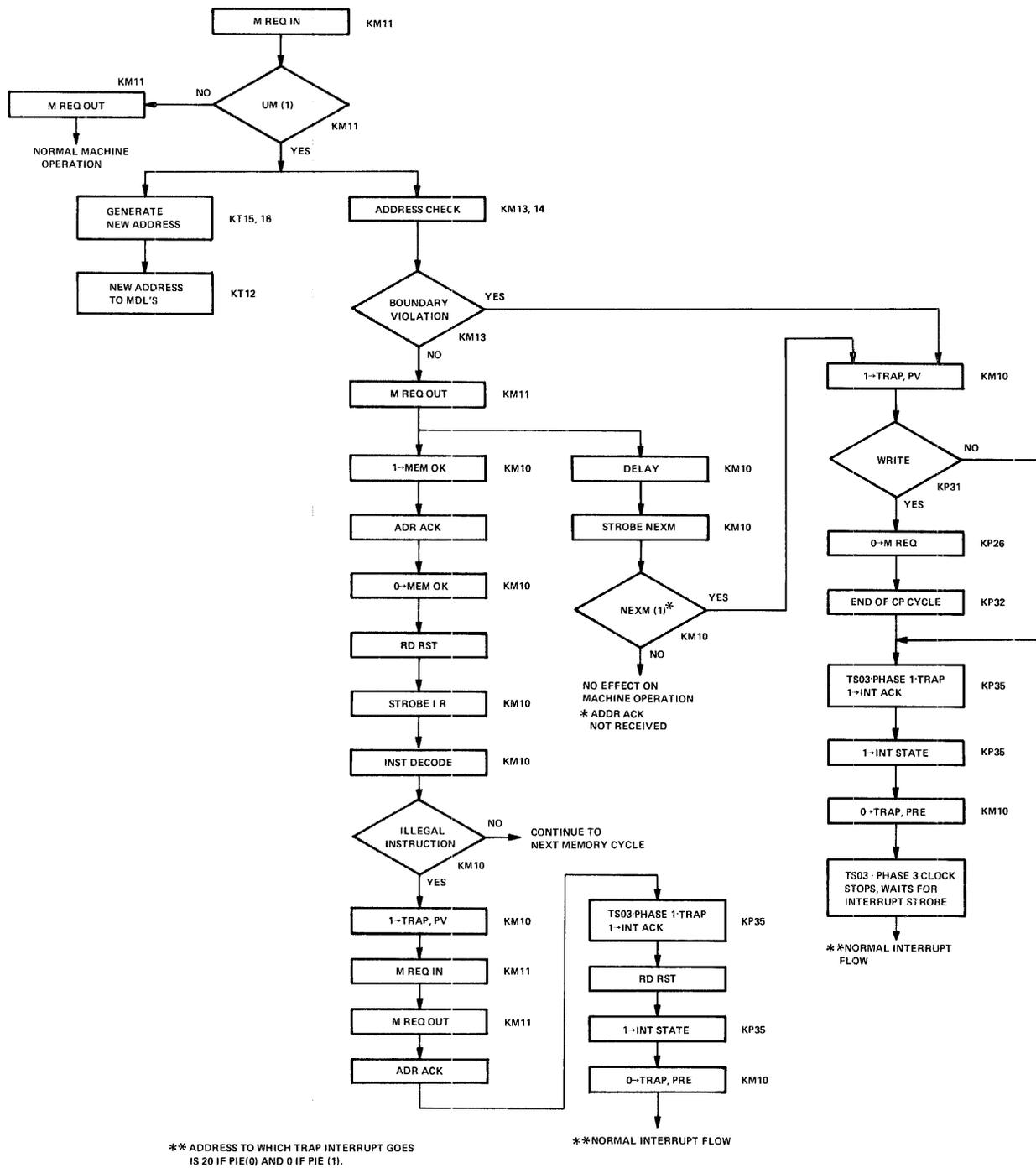
Figure 6-13 KT15 Memory Protect/Relocate Flow Diagram
