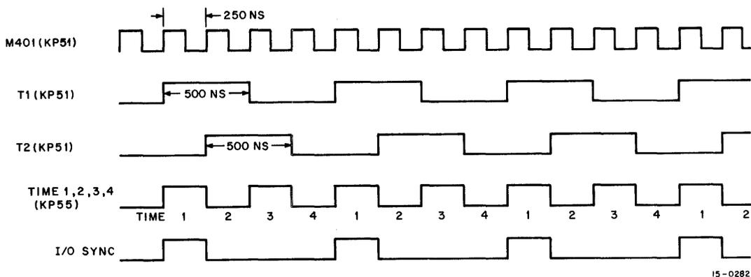
Figure 4-1 Basic I/O Timing
