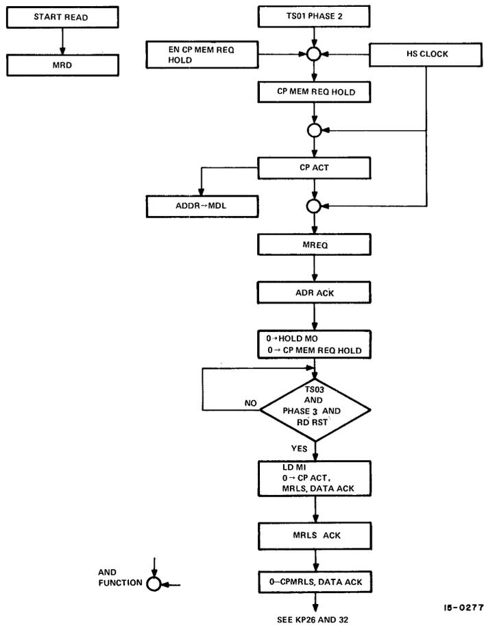
Figure 2-6 Central Processor Read Cycle
