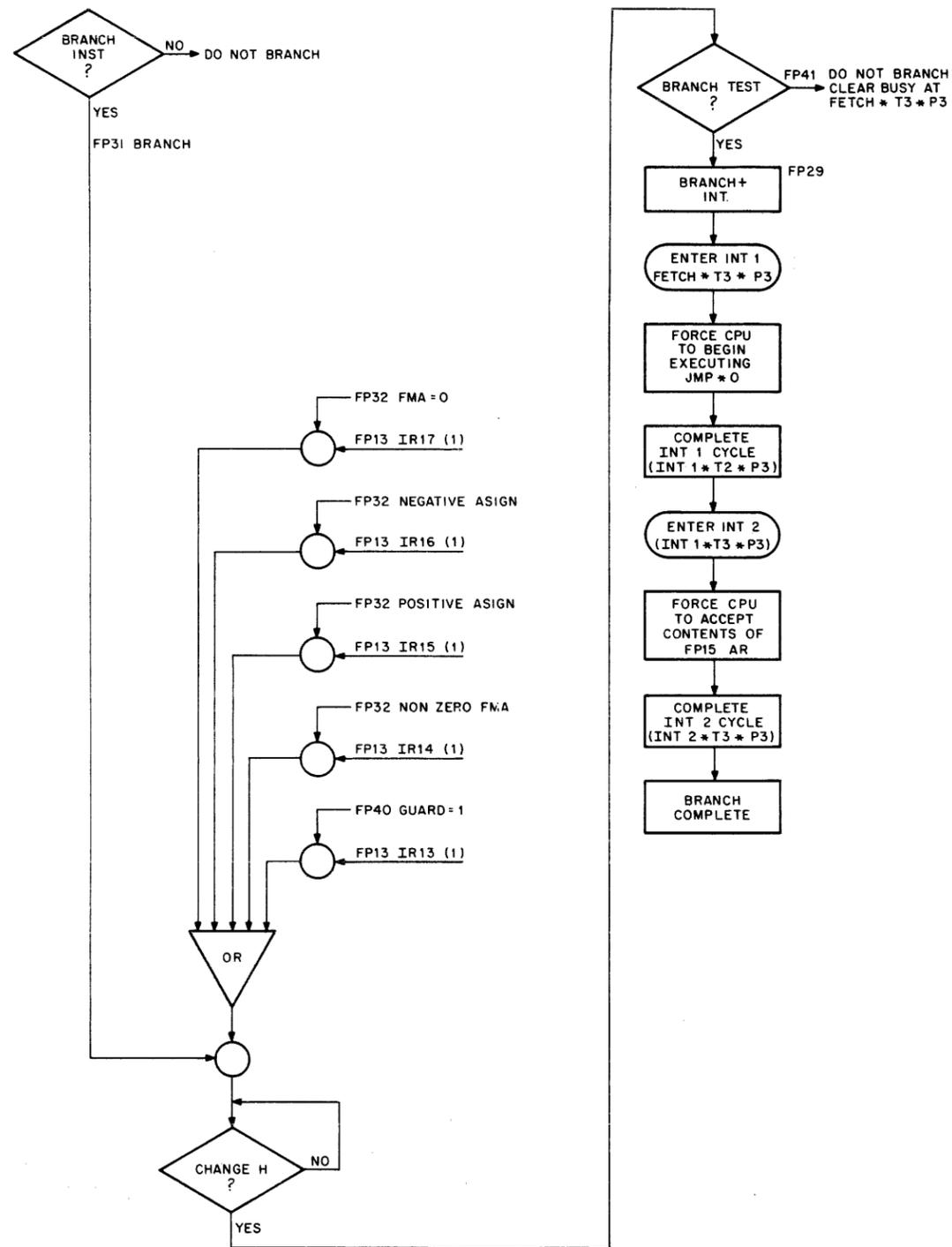
Figure 4-9 Branch Instruction Flow Diagram
