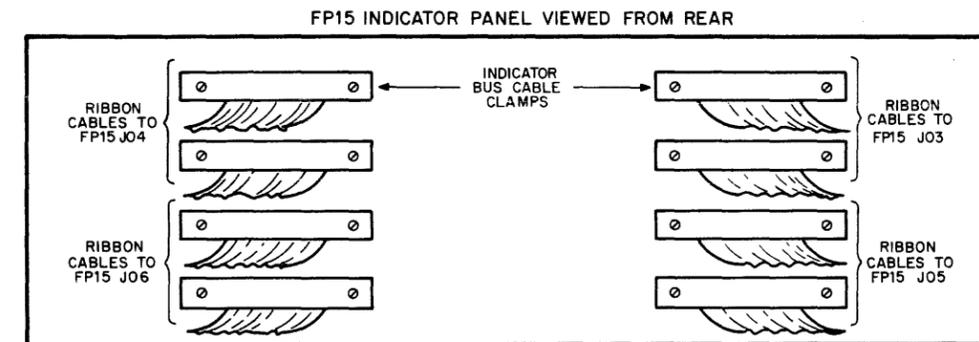
Figure 5-2 FP15 Indicator Bus Connections
