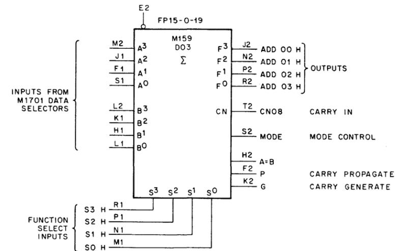
Figure 2-2 M159 Arithmetic Logic Unit
