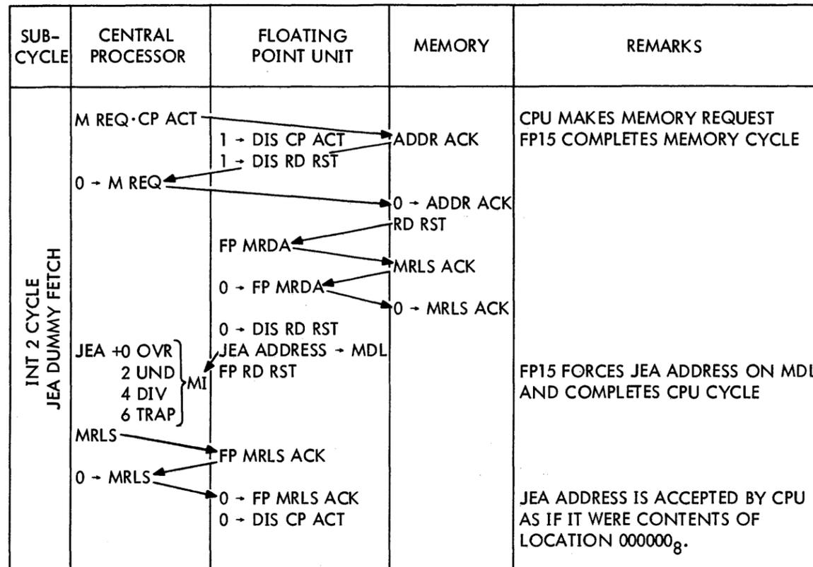
Figure 3-6 INT 2 Cycle Interface Diagram
