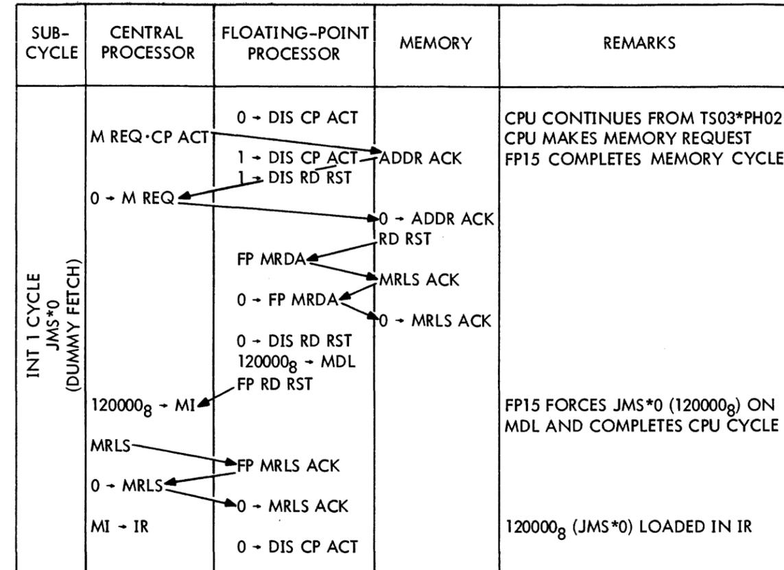
Figure 3-5 INT 1 Cycle Interface Diagram
