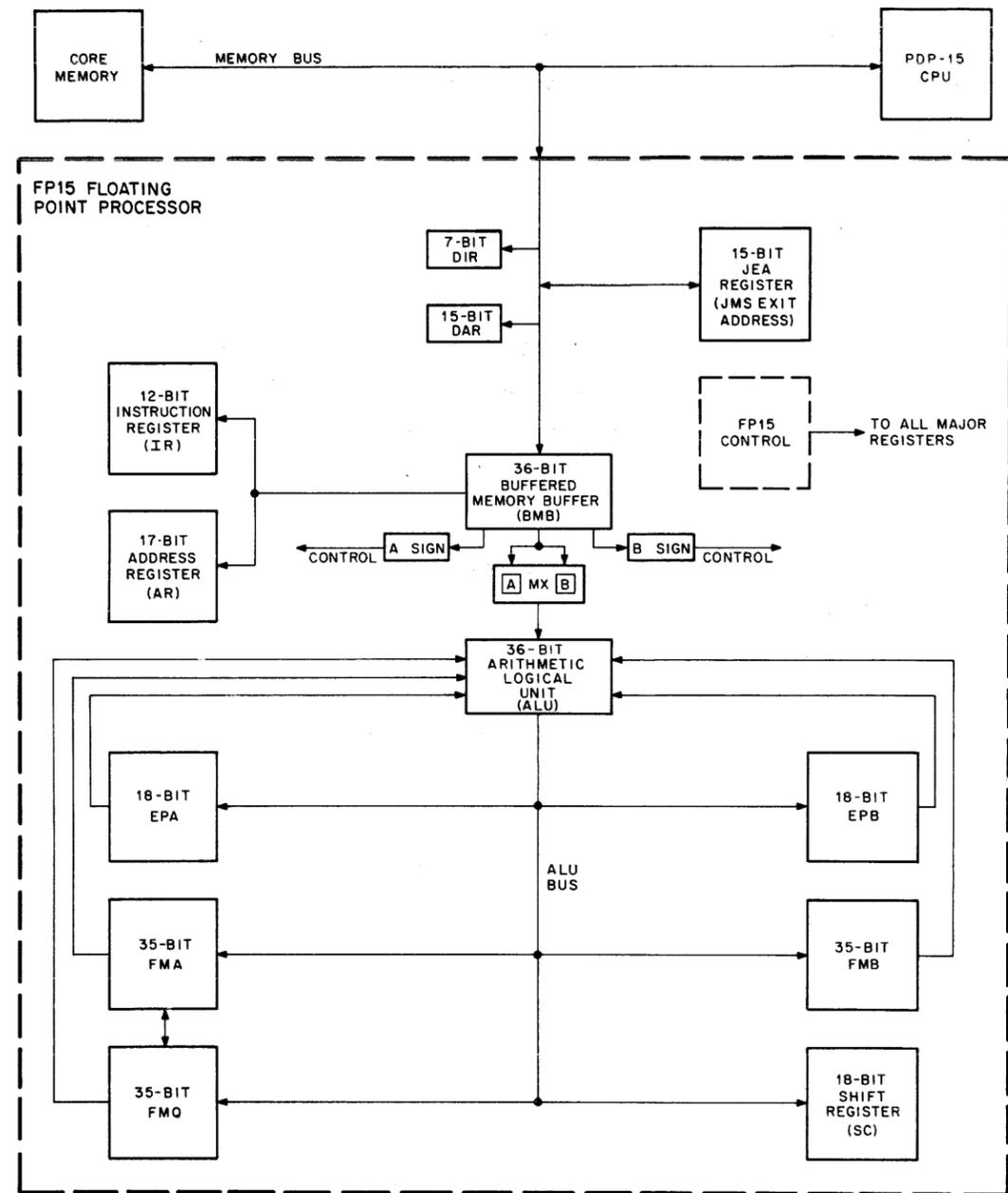
Figure 1-3 FP15 Functional Block Diagram
