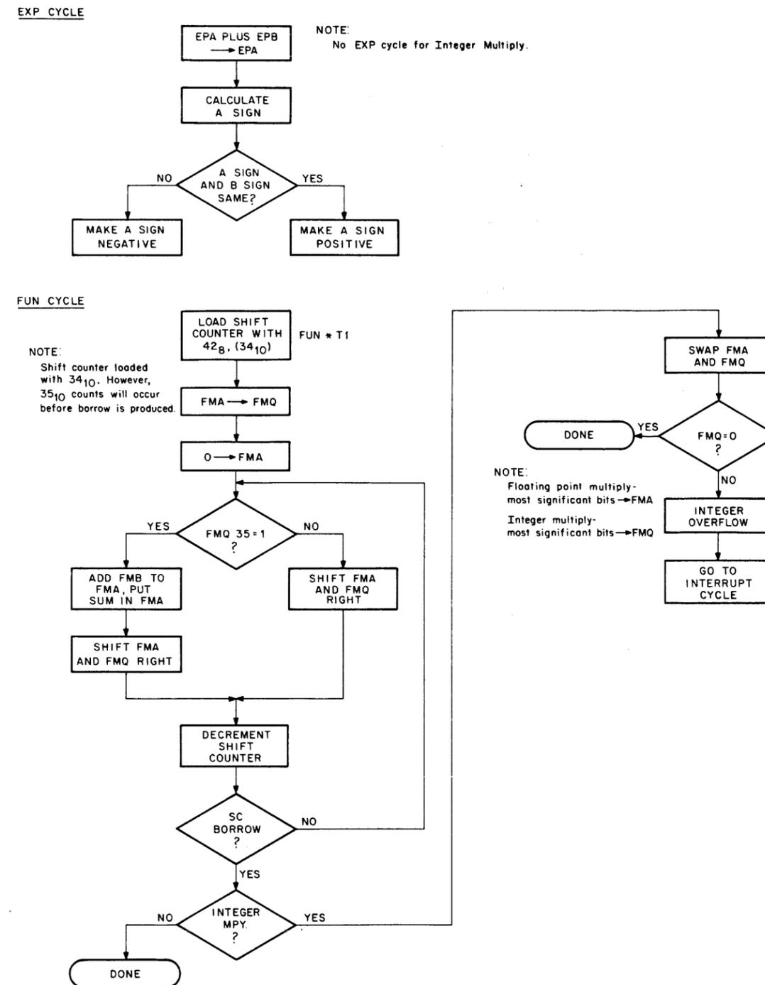
Figure 4-4 Multiply Simplified Flow Diagram
