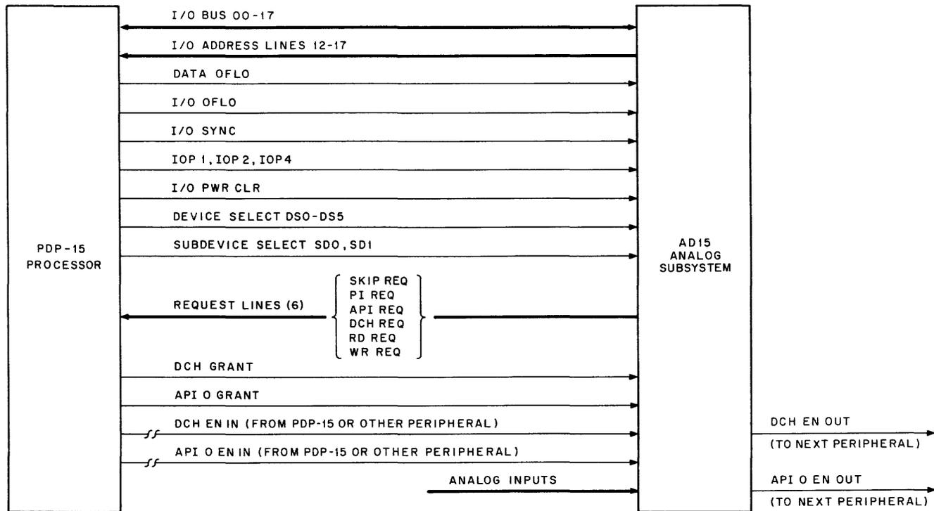
Figure 1-1 AD15 Signal Interface Diagram
