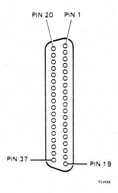
Figure C-2 37-Way D-Type Connector (Male)
