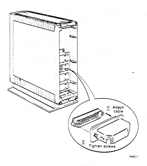
Step 2: Connect the Adapter Cable to the Extension Cable
