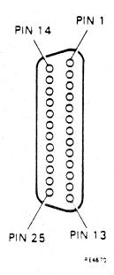
Figure C-4 25-Way D-Type Connector (Male)
