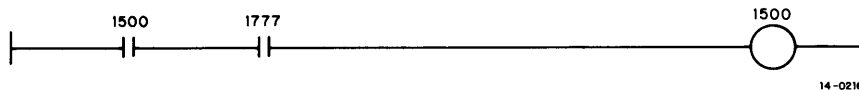
Figure 2-18 Circuit to Clear One Bit of a Shift Register on Power Failure
