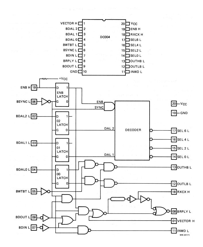
Figure C-2 DC004 Simplified Logic Diagram
