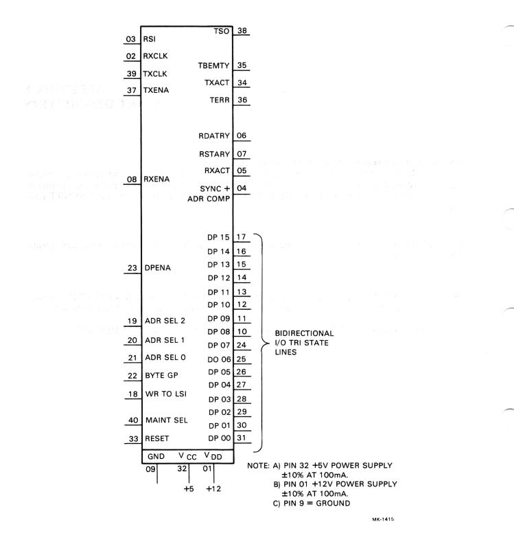
Figure B-1 Terminal Connection Identification Diagram (2112517-0-0 Variation)
