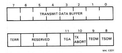
Figure 3-6 Transmit Data and Status Register (TDSR) Format
