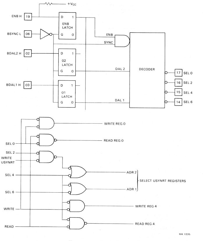
Figure 4-3 Register Decode
