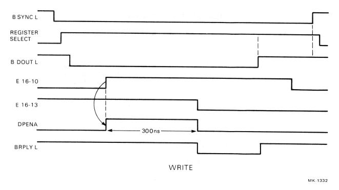
Figure 4-5 Timing for Write Operation
