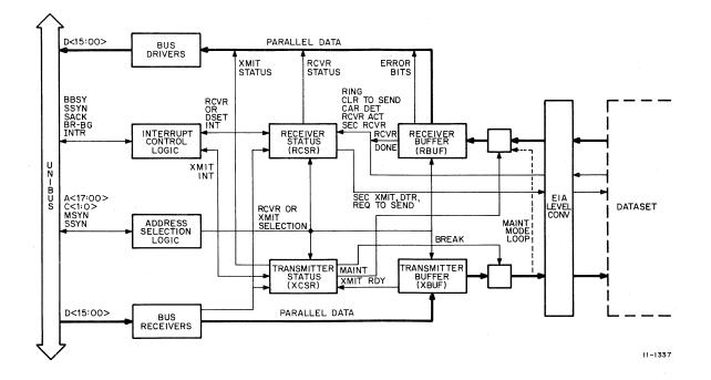
Figure 2-2 DL11-E Block Diagram
