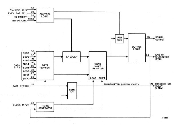
Figure 5-6 UART Transmitter – Block Diagram
