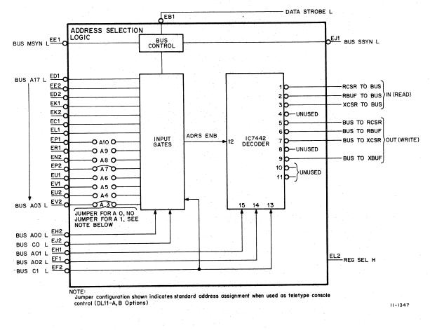
Figure 5-1 Address Selection Logic – Simplified Diagram
