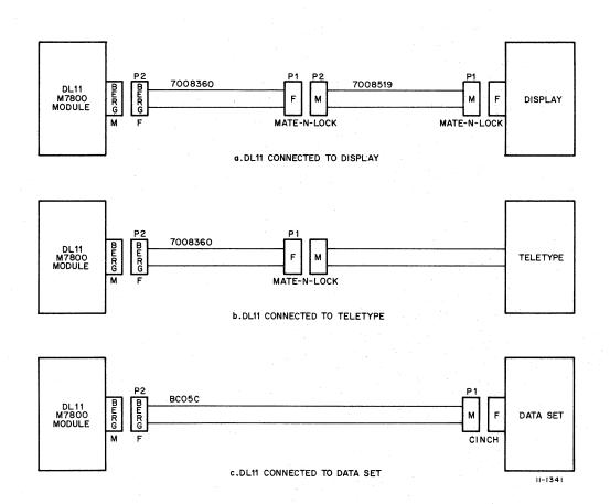
Figure 3-3 DL11 Cable Connections
