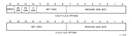
Figure 4-2 Receiver Buffer Register (RBUF) – Bit Assignments
