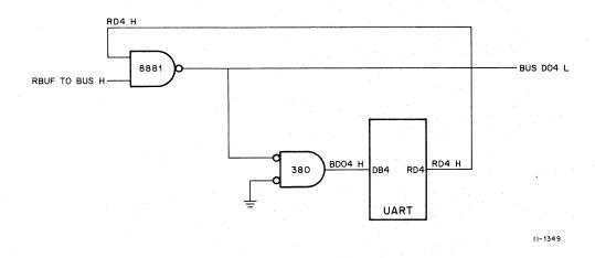
Figure 5-4 RBUF and XBUF Gating Logic – Simplified Diagram (one bit position)
