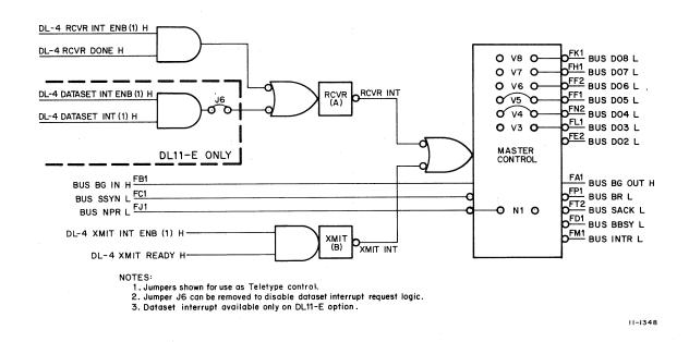
Figure 5-3 Interrupt Control Logic – Simplified Diagram
