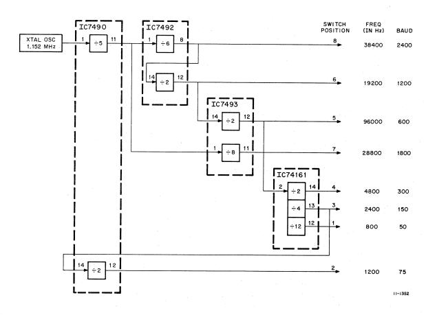
Figure 5-7 Frequency Divider Logic – Simplified Diagram
