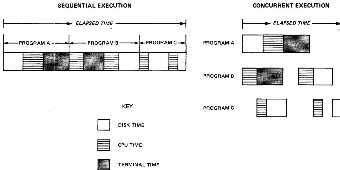
Figure 3-1 Comparison of Sequential and Concurrent Execution of Programs
