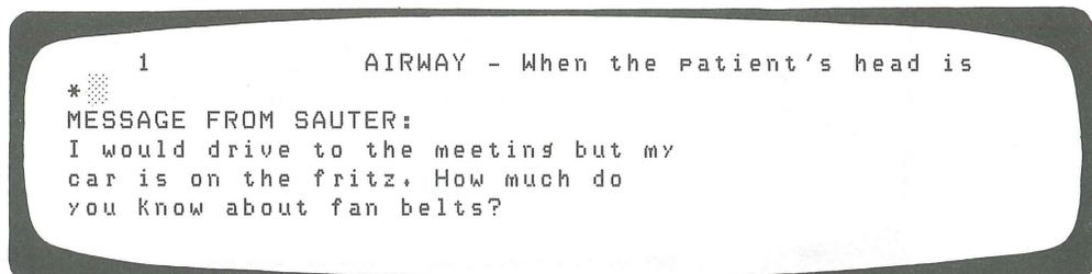
Although the message affects the display of the text, it does not become part of the buffer, even if you were inserting text at the time. You can either ignore the message or, if it bothers you, use a range specification to redisplay that part of the buffer:
